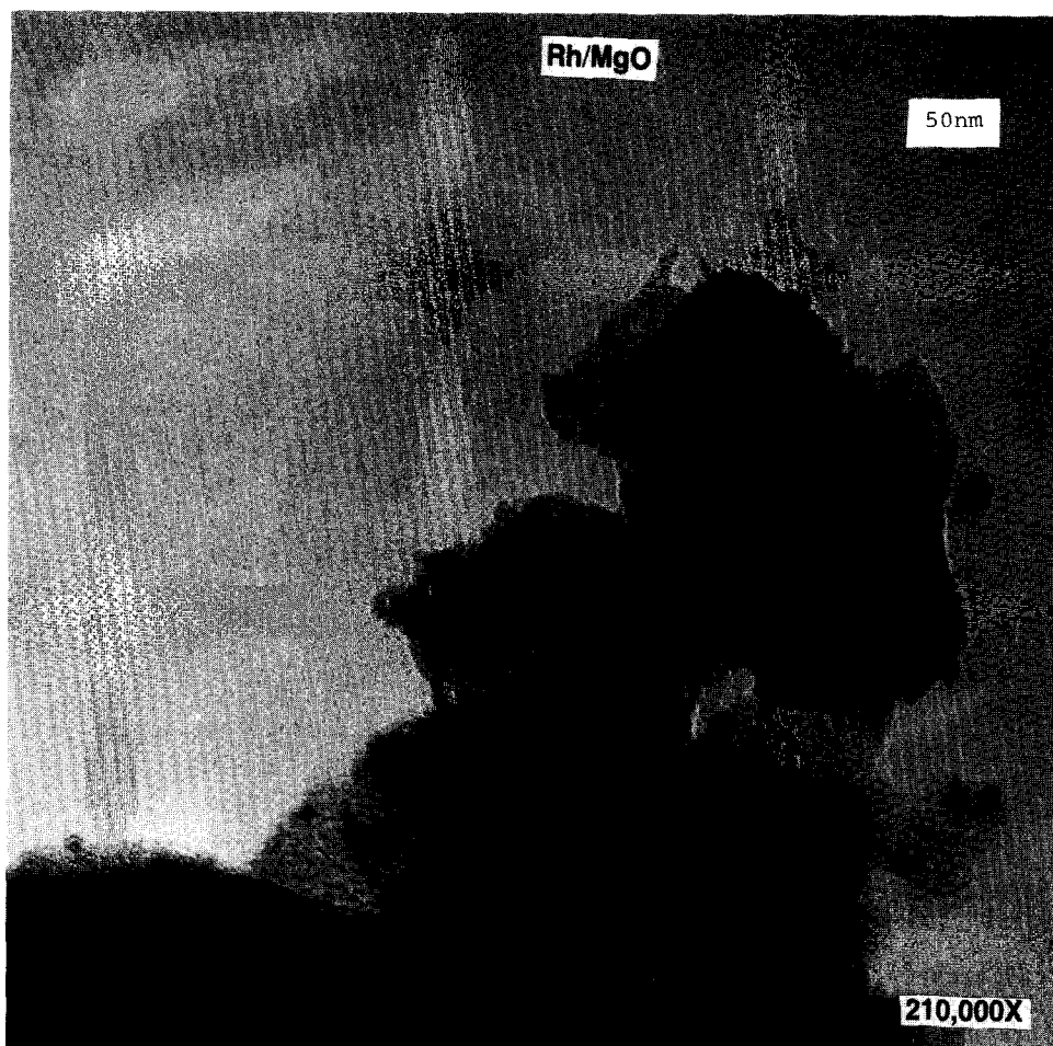
FIG. 2. TEM of rhodium on magnesia reduced at 400°C.
